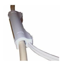
The Verticasa Breakout Unit -2 Port is typically used in multi dwelling units to breakout and distribute the fibres from an in-line Verticasa cable into a drop tube, for routing to a customer premise. It has the capacity to accommodate Verticasa cables of up to 15mm in diameter. It enables a window to be cut in the cable to access the fibres, which can be spurred of into a drop tube of 5mm in diameter.
