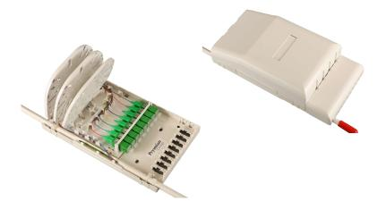
The PBI-8SC is a riser box designed for use within apartment blocks and mid/high rise office blocks. The unit houses three splice trays and up to 8 SC type pigtails and adapters. Each splice tray is able to accommodate 12 fibre splices. An in-line cable entry port enables the box to be installed onto an in-line riser cable and up to 24 drop ports are available for drop cables of up to 5mm in diameter.
