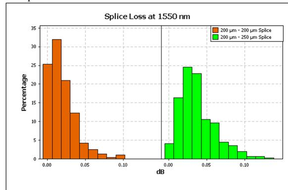
**Figure 7. Splice loss measurements for 200/200 micron OD splicing and 200/250 micron OD splicing.**
