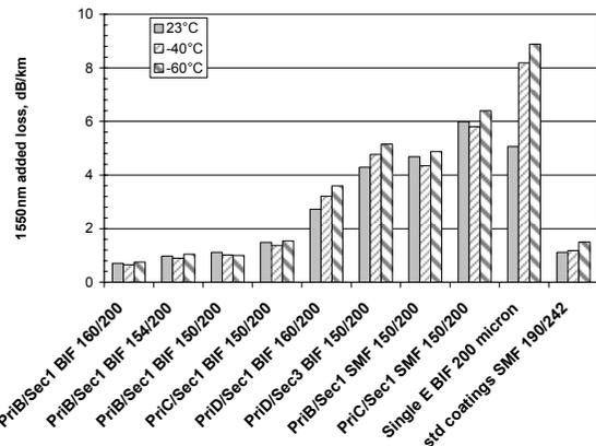
**Figure 2. 1550 nm added loss due to microbending in TR62221, fixed diameter sandpaper drum test.**
