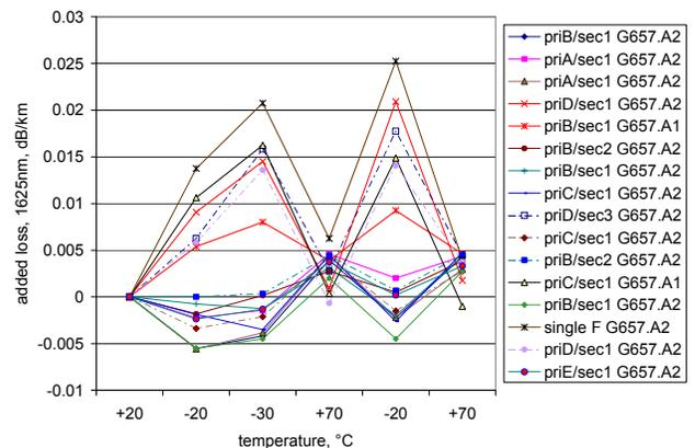
**Figure 4. Added loss at 1625nm during thermal cycling of a 720 fiber micro-module cable made with 200 micron optical fibers**
