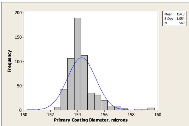
**Figure 6. Distribution of primary diameter in an industrialized process for 200 micron fiber.**
