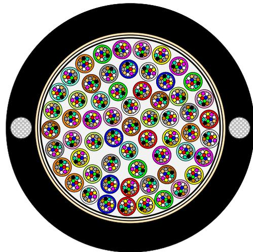
**Figure 3. Schematic of 720 fiber micro-module cable made with 200 micron fibers**
