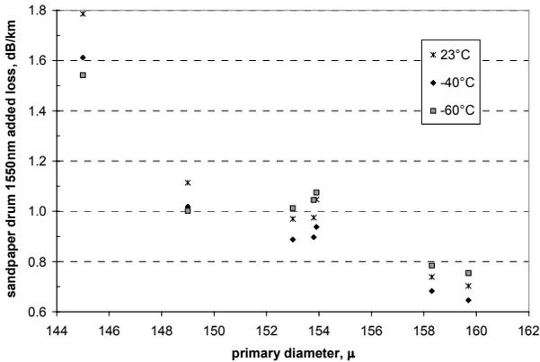
**Figure 5. Added loss at 1550nm in the TR62221.B sandpaper drum test for microbending sensitivity.**
