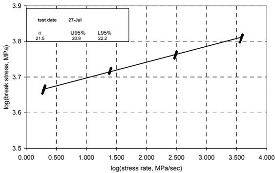
**Figure 9. Typical dynamic fatigue plot for the 200 micron coated fiber.**
