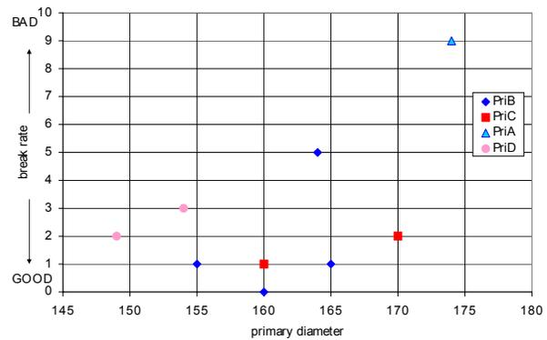
**Figure 1. Handling evaluation – removing fibers from buffer tubes and manually cleaning**
