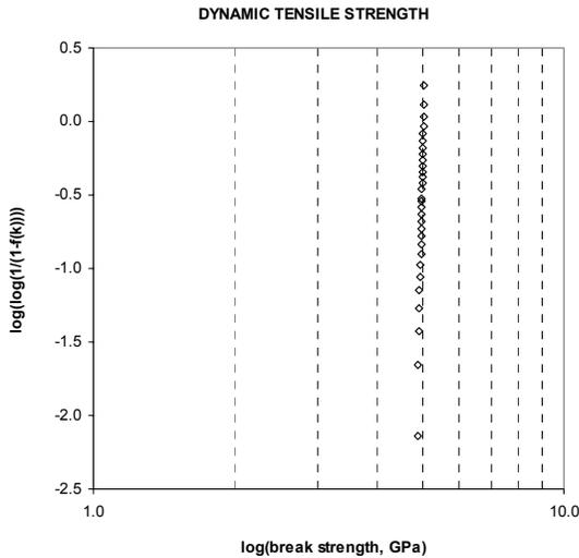
**Figure 8. Typical Weibull plot of the 0.5 meter tensile strength distribution of the 200 micron coated G.657.A2 fiber**
