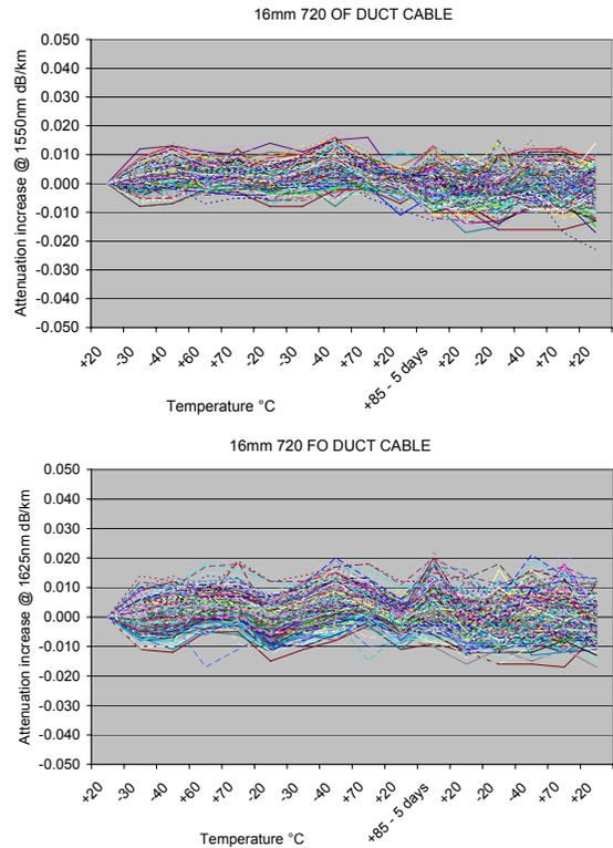
**Figure 10. Thermal cycling results on a 720 fiber micro-module cable, 1550nm and 1625nm, 180 fibers monitored in the cable.**
