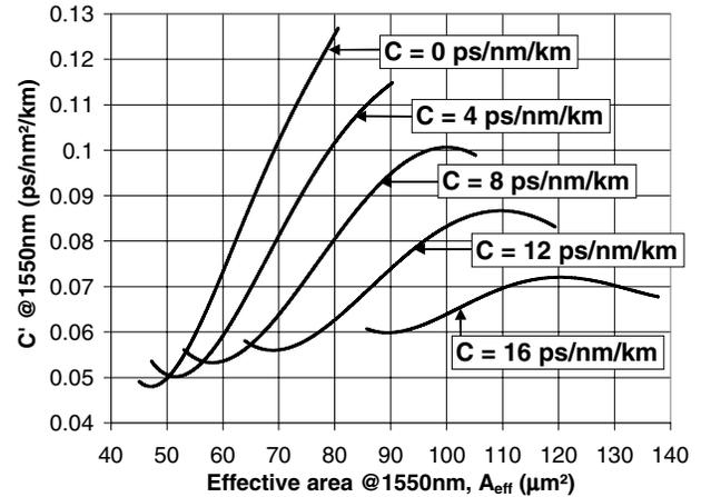
**Figure 6. Chromatic dispersion slope as a function of effective area for a set of chromatic dispersion Targets (0, 4, 8, 12 and 16 ps/nm/km), constant  $\lambda_c$  and bending loss @ 1550 nm (ensuring production of fibers with a good behavior in cable).**
