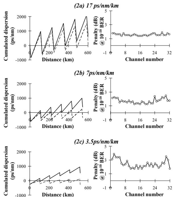
Figure 2. Best maps obtained after dispersion management optimisation and corresponding channel penalties for a  $10^{-10}$  BER, for various values of fibre dispersion at 1550 nm.
