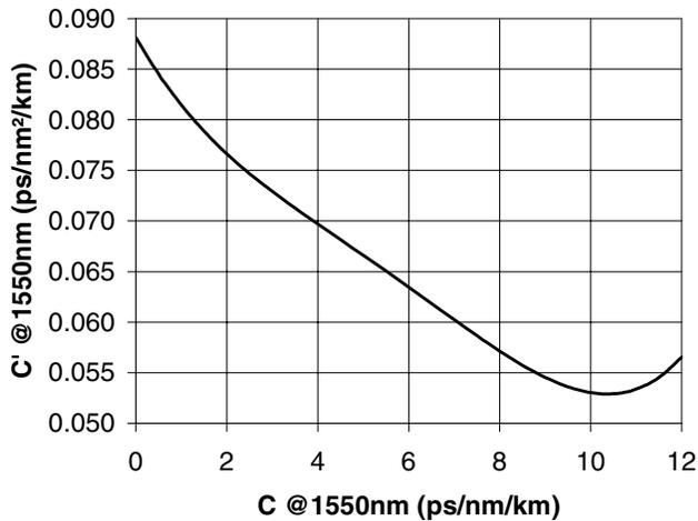
**Figure 7. Chromatic dispersion slope as a function of chromatic dispersion for an effective area of 65  $\mu\text{m}^2$ , constant  $\lambda_c$  and bending loss @1550 nm (ensuring production of fibers with a good behavior in cable).**
