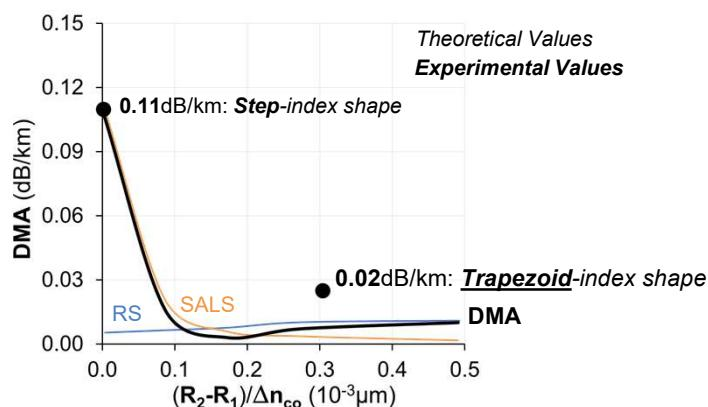
**RS:** Slightly increases because of higher  $\Delta n_{core}$  required to maintain high  $\Delta n_{eff}$
