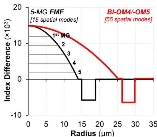
OM4/OM5 preforms can be rescaled to reach **Core radius of 14 μm on fiber to guide 5 MGs**, targeting a **diameter** that is  $25/14=1.77 \times$  larger\*
