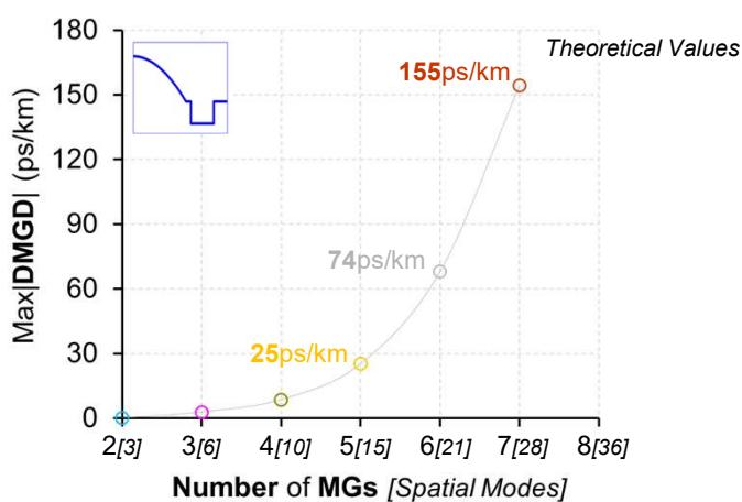
**DMGDs increase** due to the higher Core indexes\*: **critical levels are reached**
