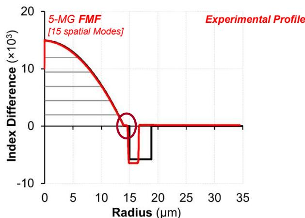
Trench-Core distance to be adjusted to further reduce **DMGDS\***
