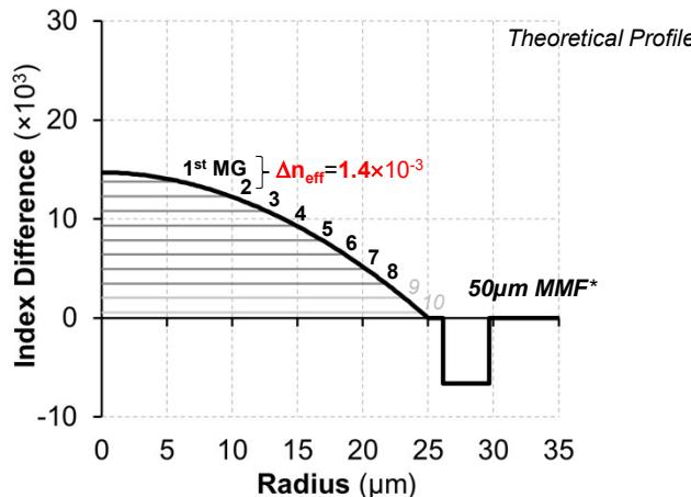
$\Delta n_{\text{eff}} > 1.4 \times 10^{-3}$ : weak coupling between last MG used and 1<sup>st</sup> MG not used
