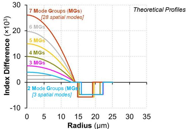
**Graded-index Core to minimize DMGDs** (as for MMFs)
