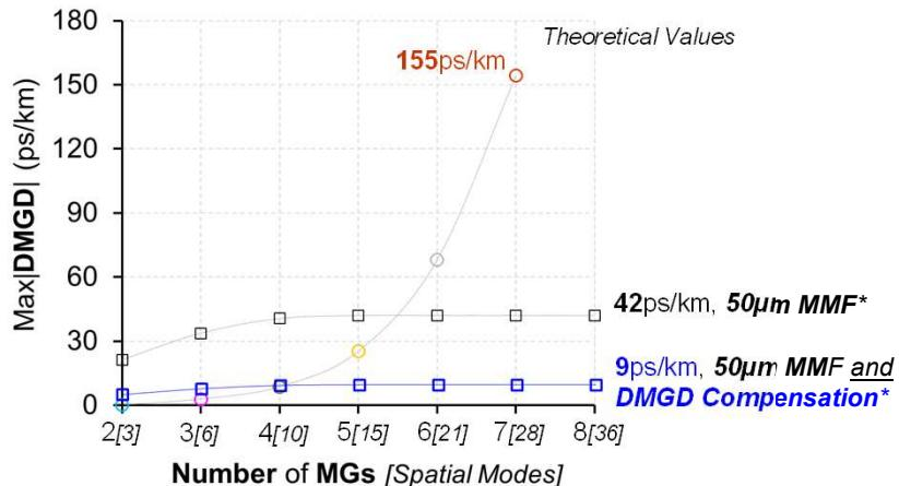
DMGDs increase due to the higher Core indexes: **critical levels are reached**
