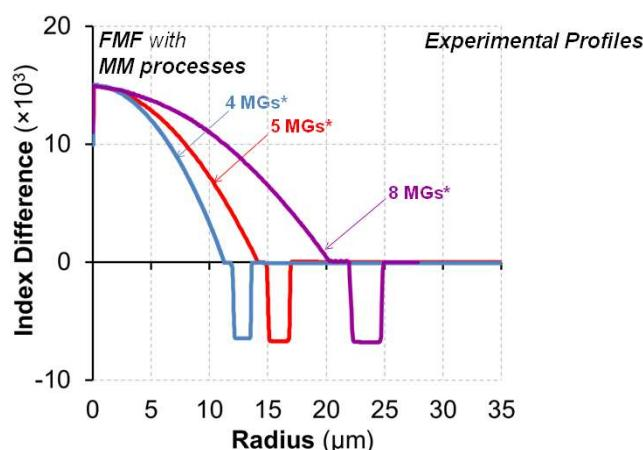
**OM4/OM5 preforms** can be rescaled to reach **Core radii** from **11.25** to **20.5 $\mu\text{m}$**  on fiber to guide **4 to 8 MGs** [10 to 36 spatial modes]
