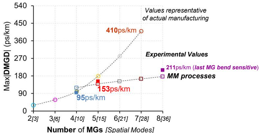
**DMGDs calculated from distributions of profiles with  $\sigma$  that match process tolerances:** representative of manufacturing
