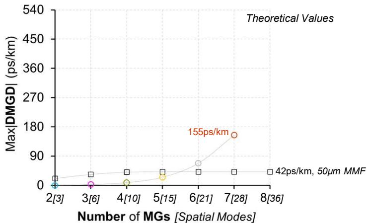
Such low **DMGDs** cannot be reached given the sensitivity to profile variations (that occur during the manufacturing)
