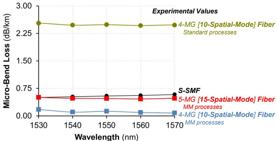
**Increasing effective index difference between guided modes and radiation/leaky modes reduces micro-bending sensitivity\***
