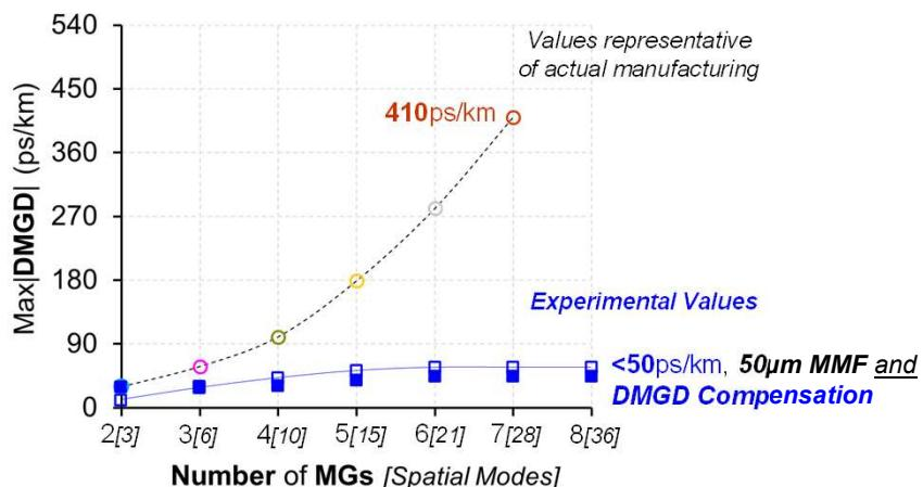
**8 MGs** considered: **9<sup>th</sup> and 10<sup>th</sup> MGs** being more bend sensitive, might not be suitable for MDM
