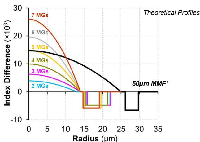
Core index of  $50\mu\text{m}$  MMF  $\leq$  Core index of MMFs with MGs  $\geq 5$
