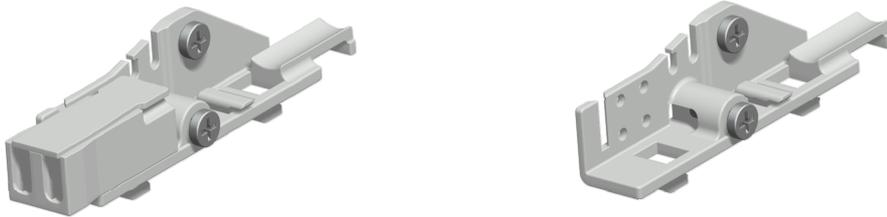
The ARS Cable Clamp is used to anchor a single cable and to distribute up to 4 cable elements (48 fibres). The ARS is suitable for cables between 12 and 48 fibres. 10 metres of routing tube is supplied with the ARS. The ARS allows for the anchoring / termination of both the cable strength member and any Aramid within the cable construction.
