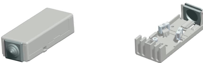
The BEM Cable Clamp is used to anchor a single cable and to distribute up to 16 cable elements (192 fibres). The BEM is suitable for cables between 36 and 192 fibres. 20 metres of routing tube is supplied with the BEM. The BEM allows for the anchoring / termination of both the cable strength member and any Aramid within the cable construction.
