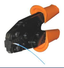
The **Verticasa Crimp Set** is used to crimp a fibre module to the pulling rope in a Verticasa drop tube, for pulling the fibre module into the customer premises. It is also used to crimp the 5mm metal crimp ring in the Verticasa Customer Connection Kit.
