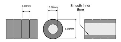
Bend Limiting Transport Tube is supplied in 10m coils for applications where routing of fibre within equipment racks and cable nodes etc is required. The Bend Limiting Tube provides excellent protection in these environments especially where resistance to crushing and kinking are required and fibre bends are limited and maintained to an acceptable radius.
