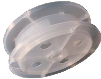
The Verticasa Storage Reel is used to temporarily store an extracted fibre module before installation into a customer drop tube. The reel ensures that the extracted fibre is kept safe from damage, and is stored to the correct bend radius. The fibre module can be simply wound onto the reel as the fibre module is extracted, and wound back off when the fibre module is ready to be installed into the drop tube.
