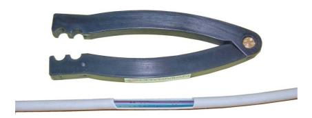
The Verticasa Cable Stripping Tool Compact (VST-C) is typically used in multi dwelling units or office fibre cabling systems where extractable fibre cables like the Prysmian Verticasa cable range have been installed. It is used to create a longitudinal window cut on the cable. The window cut will allow to access the fibre modules inside the cable.
