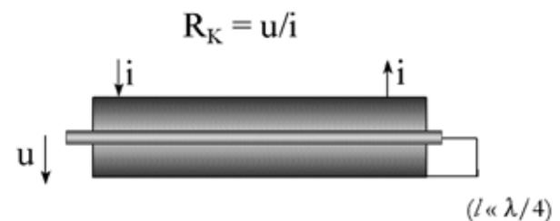
Figure 1: Definition of transfer impedance
