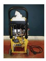
The Sirocco Compressor is designed to deliver clean, dry air for installation of Blown Fibre units using compressed air. The Sirocco Compressor is a quiet, portable, electric motor driving a reciprocating compressor unit. Producing 60 l/min (0.06m3/min, 2.1 cfm) of treated compressed air at a maximum working pressure of 8 bar, it provides the ideal source of compressed air for the installation of blown fibre units for the FTTH market.
