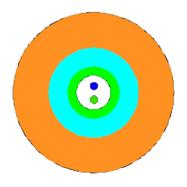
Central gel filled tube housing the BendBright fibers
