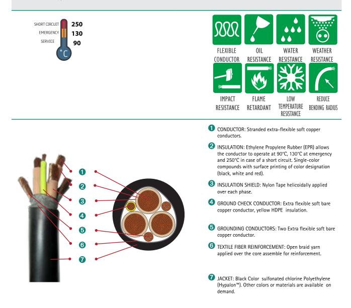
PRINT: General Cable G-GC 3x [conductor size] + 2x [grounding conductor size] +1x [ground check conductor size] AWG Cu 2 kV HECHO EN CHILE
