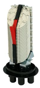
The Compact Single Circuit Joint allows the termination of up to 96 fibres (4 fibres per tray). The joint is available with either 6 circular ports or 1 oval port and 4 circular ports.
