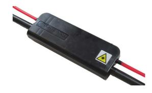
The RetractaNet<sup>xs</sup> TBE-12 Tapping Box is used to breakout and distribute the fibres from an in-line RetractaNet cable into drop tubes, for routing to a customer premises. It is sealed to IP68, enabling it to be mounted in the underground environment. It has the capacity to accommodate an in-line RetractaNet cable of up to 15mm in diameter. It enables a window to be cut in the cable to access the fibres, which can be spurred of into a drop tube of up to 7mm in diameter.
