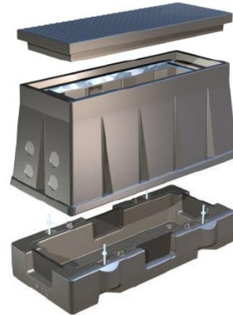
The hand hole type Z6P1-M001 is designed as a direct buried underground housing. The hand hole can be connected to a duct or cable system and supports the installation of most types of splice closures. The hand hole can be used as an underground manipulation point for micro ducts and / or fibres on all network locations. The hand hole has separate bottom part to enable installation over existing ducts or cables. The hand hole opening is reinforced with a metal frame.
