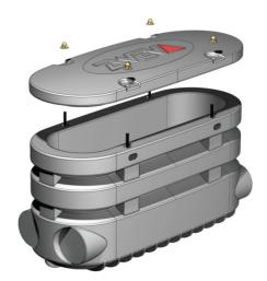
The hand hole type ZTTH3-P001 is designed as a direct buried underground housing. The hand hole can be connected to a duct or cable system and supports the installation of most types of splice closures. The hand hole can be used as an underground manipulation point for micro ducts and / or fibres on all network locations. is designed as a direct buried underground housing.
