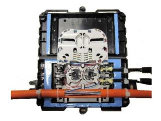
The TBE-I4 Tapping Box is used to distribute the fibres from an in-line Retractanet cable into drop cables, for routing to a customer premises. It is sealed to IP68, enabling it to be mounted in the undergorund environment. It has the capacity to accommodate an in-line cable of up to 13mm in diameter. The closure also provides the facility to accommodate sixteen fusion splices. The closure is re-enterable and can be supplied in grey or black.
