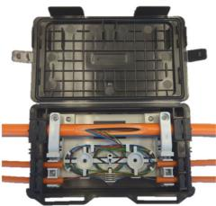
The RetractaNet<sup>xs</sup> TBE-I4 ST Tapping Box is used to breakout and distribute the fibres from an in-line Retractanet cable into drop tubes, for routing to a customer premises. It can be mounted in the outdoor environment, and has the capacity to accommodate an in-line Retractanet cable of up to 15 mm in diameter. It enables a window to be cut in the cable to access the fibres, which can be spurred of into maximum 4 drop tubes of 6 to 7mm in diameter.
