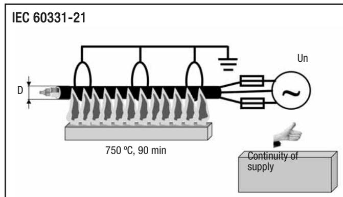
Fire resistance attempts to show the capacity of the cable to provide service in extreme fire conditions. Fire resistant cables are used for services which are intended to continue to function in case of fire (security and indispensable services).
