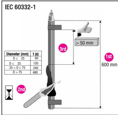
The flame retardancy test (IEC 60332-1) consists in checking the fireproofing of a single simple of cable in vertical position. Depending on the outer diameter of the cable, the flame is applied for between 1 and 8 minutes. The test is considered passed if fire does not affect the cable past the last 5 cm. The spread of flame is also limited towards below the fire.
