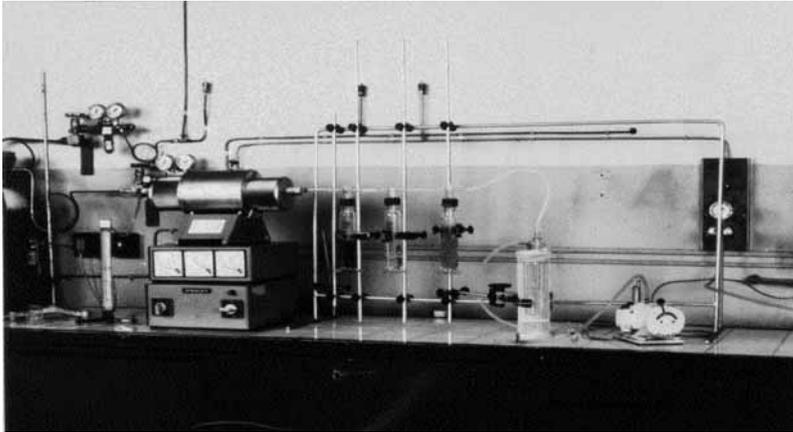
These two similar tests demonstrate that the cable tested is halogen free (does not emit HCl or other halogenated composites in combustion) and that the gases emitted are of very low corrosiveness, with the aim of protecting people and property in case of fire.
