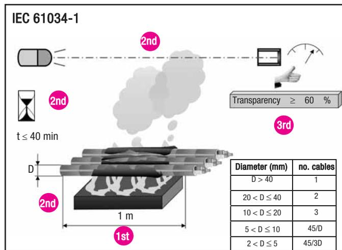
The opacity of smoke produced by fires is an important factor to be considered when the occupants of a site must evacuate it in the first moments, even if extinction and rescue teams are to take action a few minutes later in the premises affected by the accident.
