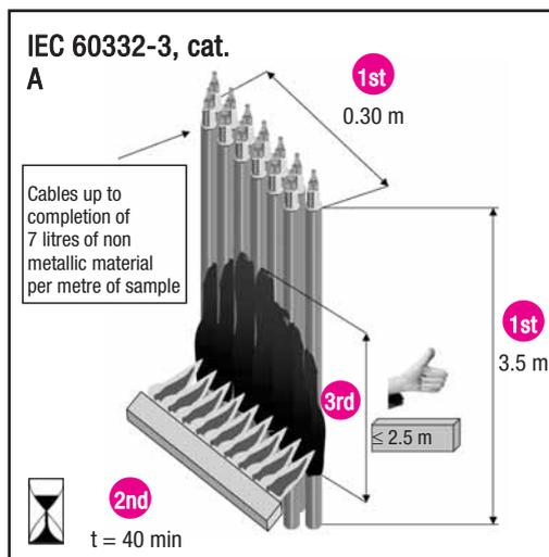
Cables are normally grouped in the cable runs, making it necessary to check behaviour in fire conditions in group. In the fire retardancy test, (IEC 60332-3, category A) samples of 3.5 m of a determined section are grouped to completion of until 7 litres of non metallic material per metro of sample. They are subjected to the action of flames for 40 minutes. If the final length affected by fire is less than 2.5 m, the test is considered as passed.
