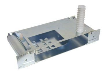
The Generic Sub-Rack 3A (GSR3A) is designed for use in ETSI compliant Optical Equipment Racks. The GSR must be used in conjunction with a Rack Splicing Module. The maximum capacity of the GSR3A is **48** spliced fibres (one RSM), based on single circuit management.
