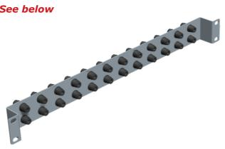
The Sirocco Blown Fibre Tube patching Panel is compatible with 19'' and ETSI rack practice. The unit provides the patching capacity for up to  $24 \times 5$ mm diameter blown fibre tubes and allows for quick and easy reconfiguration of tube routing. The unit is supplied with  $24 \times 5$ mm diameter bulkhead connectors and all accessories required to install the patching panel in to the rack.
