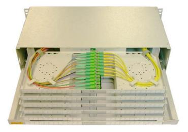
The OAsys Sliding Sub-Rack (Patching) is a 3U shelf for use within 19" and ETSI standard racks allowing the connection of up to 72 fibre patches. The shelf contains six pull out modules, which each house 12 adapters. The modules hinge upwards to provide access to the module below. The shelf is supplied with all of the adapters pre-installed at Prysmian to save installation time, and a variety of different adapter types can be accommodated.
