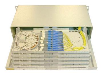
The OAsys Sliding Sub-Rack (Splicing and Patching) is a 3U shelf for use within 19" and ETSI standard racks allowing the connection of up to 72 fibres onto Adapter Panels. The shelf contains six pull out modules, which each house a splice tray and 12 adapters. The modules hinge upwards to provide access to the module below. The shelf is supplied with all of the pigtails and adapters pre-installed at Prysmian to save installation time, and a variety of different adapter types can be accommodated.
