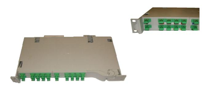
The Connectorised Splitter Shelf is a 1U plastic shelf that allows pre-connectorised splitters to be mounted onto adapter panels. The shelf is compatible with 19" and ETSI racks and can accommodate connectorised splitters from 1x2 to 1x32 configurations, using SC or LC connectors. The shelf is supplied with the splitters pre-installed by Prysmian with both input and output fibres from the splitter being connectorised which makes patching splitters into networks extremely easy.
