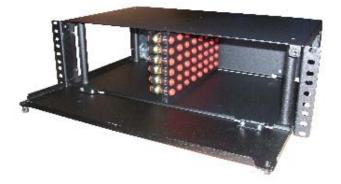
The 19" Blown Tube Patch Shelf provides a solution for connecting up to 48 blown fibre tubes of 5mm in diameter. The shelf is 3U in height and can be mounted into a 19" rack or street-side cabinet. The connectors inside the shelf are gas block connectors which means the shelf is ideal for connecting external tubes to internal tubes. The unit is supplied with the 48 gas block connectors mounted into the steelwork and the fixings required to install it into a rack or street-side cabinet.
