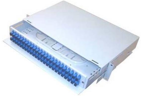
The DOBEX-2U Distribution Drawer is a 2U splice and patch panel for installation into 19" or ETSI racks. The product is fully metallic and has a capacity of up to 96 fibres on a splice and patch basis. The product can be configured with FC, ST, E2000, SC or LC type pigtailed and adapters..
