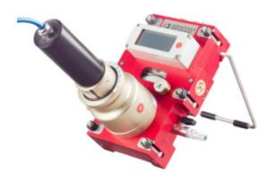
The Sirocco Blowing Head is designed for the installation of Enhanced Performance Fibre Units (EPFU) into tubes using compressed air. The Sirocco Blowing Head is used in conjunction with a compressor (petrol or electric, see datasheets SI002 and SI003 respectively) that provides clean, dry, technically oil-free air at 10-bar to propel the fibre unit through the tube. Installation speed, which is controlled by the clutch system, is a maximum 50 m/min.
