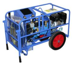
The Sirocco Compressor is designed to deliver clean, dry air for installation of optical fibre using the blown fibre technique.
