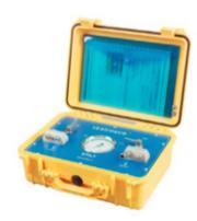
The patented Sirocco Tube Integrity & Length Tester (STILT) will enable installers of the Prysmian Sirocco blown fibre solution to ensure that the link (tubes and connectors) to be used to install EPFU is free from any air leaks and that there is an adequate length of blown fibre unit available to complete the installation.
