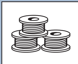
Upended heavy reels will often arrive damaged. Refuse or receive subject to inspection for hidden damage.
