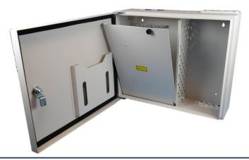
Termination box PK-300 is a metallic cabinet with a lockable door. Termination Box PK-300 is designed for the termination and distribution of various types of fibre optic cables in indoor installations. Termination box is wall-mountable and dust-proof. A patch panel divides the box into splicing and cross-connection sections.
