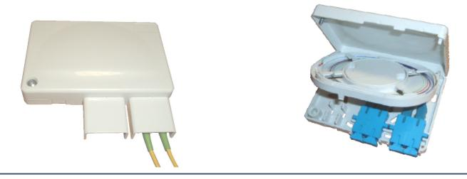
The Compact Termination Box is designed for use in residential and business applications for the termination of up to four optical fibres. The wall box enables the installation of either a single Blown Fibre Tube Cable with up to a 4 fibre blown fibre unit installed <u>or</u> up to two 2 fibre ruggedised cables to be spliced to four SC pigtails (PC or APC).
