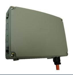
The External Customer Splice Box is designed for use on the external wall of residential or small business premises. The unit houses a single splice tray and allows fibre from externally fed cables (Blown Fibre or standard cable) to be spliced to pigtails for connection to adapters. Patch-cords are routed through the external wall fabric into the premises via a rear exit port. The unit can also be used as a transition point between internal and external cable (or ruggedised pigtails).
