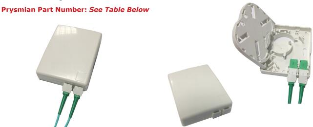
The Ultra Compact Termination Box is designed for use in residential and business applications for the termination of up to two fibres. The wall box enables the installation of a small cable to be spliced to up to two SC pigtails (PC or APC), which connect to shuttered adapters at the base of the unit. The unit can be quickly installed within an office, house or communication room environment.
