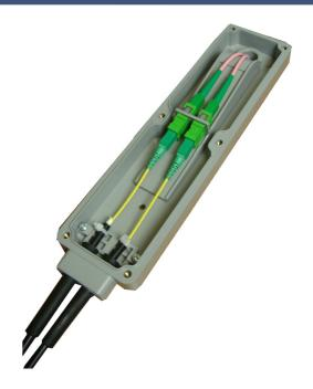
The QUICKDR@W Demarcation Unit enables up to two QUICKDR@W cable Lead In Assemblies to be terminated on the outside wall of a building. It provides a connection on the external wall for test and maintenance access. Patch-cords can then be passed, fully bend managed, through the wall into the building for connection to active FTTH equipment. The unit is sealed to prevent the ingress of moisture to IP55.
