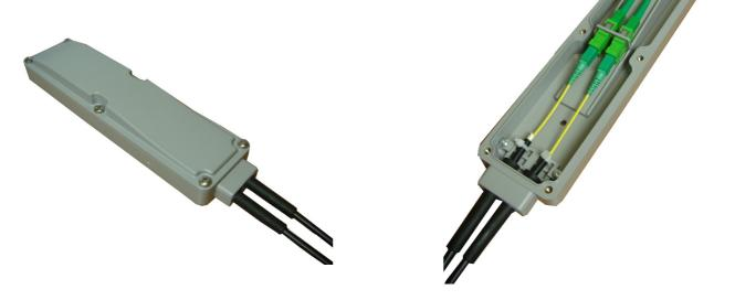
The QUICKDR@W Demarcation Unit enables up to two QUICKDR@W cable Lead In Assemblies to be terminated on the outside wall of a building. It provides a connection on the external wall for test and maintenance access. Patch-cords can then be passed, fully bend managed, through the wall into the building for connection to active FTTH equipment. The unit is sealed to prevent the ingress of moisture to IP55.
