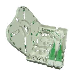
The MK2 Ultra Compact Termination Box is designed for use in residential and business applications for the termination of up to two fibres. The wall box enables the installation of a small cable to be spliced to up to two SC pigtails (PC or APC), which connect to shuttered adapters at the base of the unit. The unit can be quickly installed within an office, house or communication room environment.
