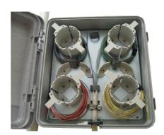
The Verticasa Top Loop Box is a secured box allowing the coiling of extra lengths of Verticasa fibre modules. The box does not contain any splice trays and is used purely to coil the overlength of fibre modules at the top of a Verticasa riser cable. The box is wall mountable and is for internal use. The box enables one cable of up to 15mm to enter.
